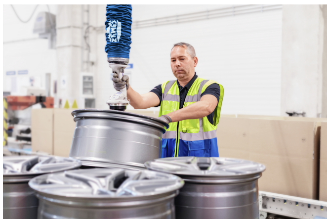
The rim gripper for JumboFlex vacuum tube lifters handles heavy rims with ease.
