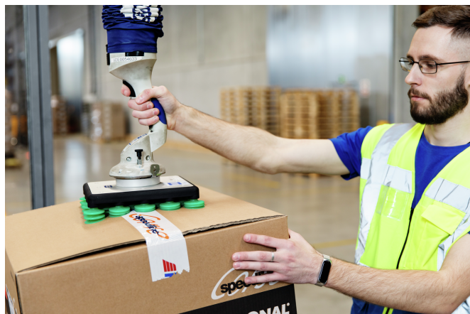
The JumboFlex tube lifter with multiple grippers picks up cardboard boxes of different sizes and qualities safely.
